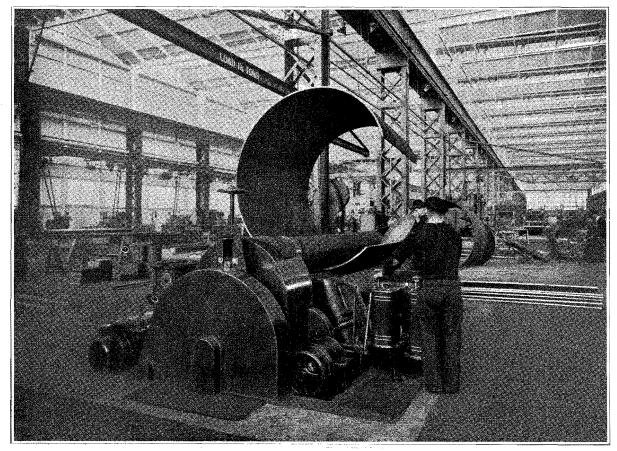
BENDING AND STRAIGHTENING HORIZONTAL ROLLS, Boiler Shop, Newport Workshops.
